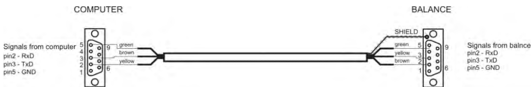
Balance - computer cable (RS232)
