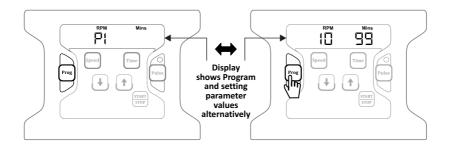
Press the "Program" button to select any program from "P1 to P9". Programs can also be select by pressing "Increment or decrement" button. Once require program is selected, press the "speed button" to select and set speed value. Press "Time" to select and set time value.
